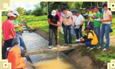
JICA Expert Mr. Takamitsu Matsuo demonstrates the use of current meter in a session of the Water Flow Monitoring Method training for NIA O&M staff and selected farmer-leaders in Mambusao RIS (Region 6).
